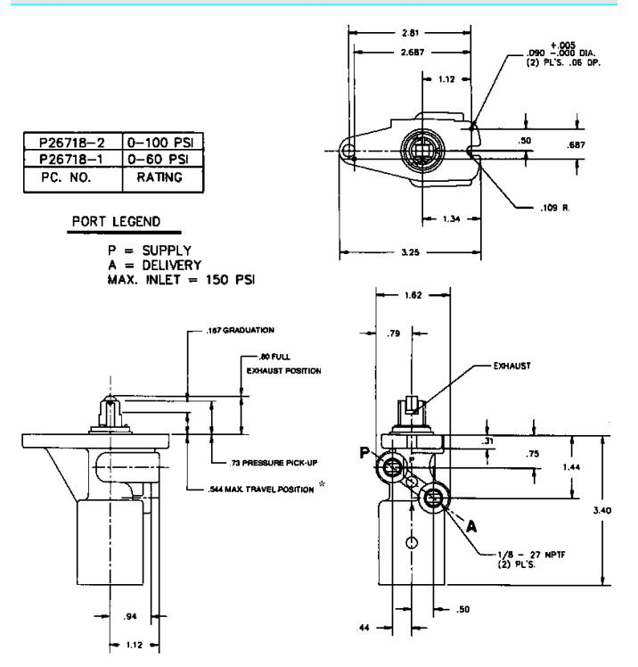
\*Travel beyond this position can result in over pressure with possible valve damage.
